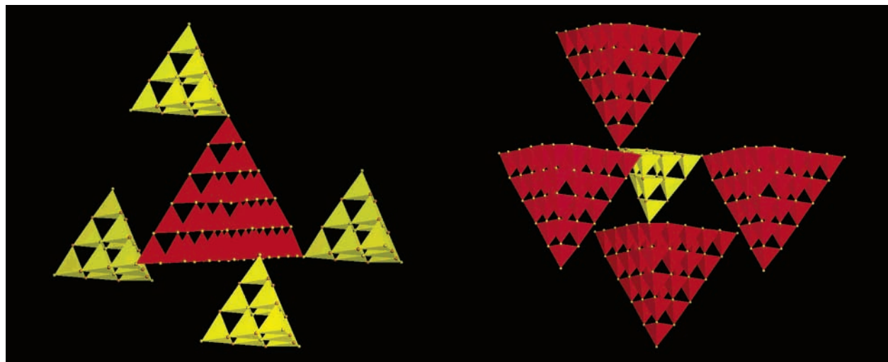
FIGURE 5. In UCR-15, four T3 clusters ( In_{10}S_{18}^{6-} ) are joined together by a pseudo-T5 cluster ( In_{34}S_{54}^{6-} ) and vice versa.
